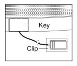
ment, the displays will light. IMPORTANT: In an emergency situation, the key can be pulled from the console, causing the walking belt to slow to a stop. Test the clip by carefully taking a few steps backward; if the key is not pulled from the console, adjust the position of the clip.
